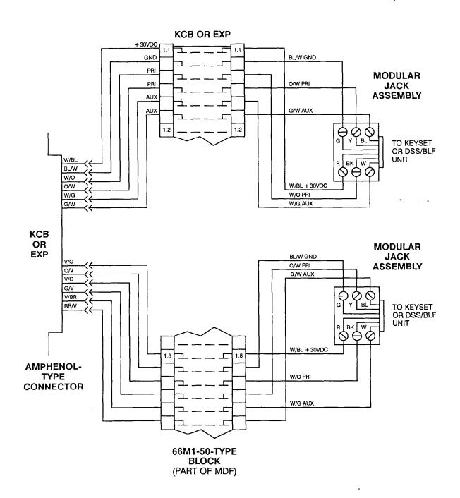
NOTE: For proper keyset operation, all three pairs (power/ground, primary, and auxiliary) are required.
