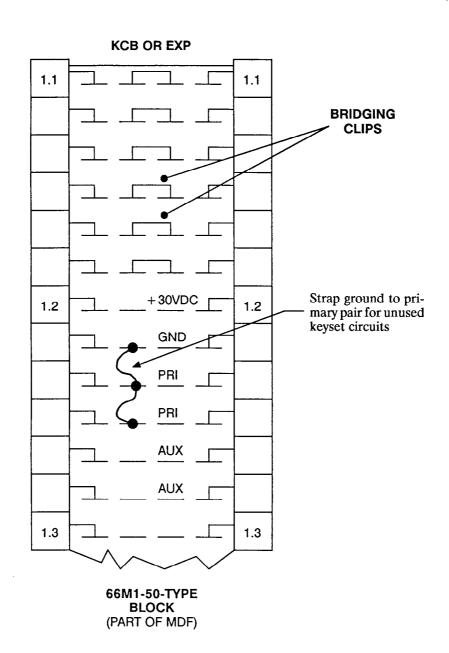
NOTE: To later install a station instrument on an unused keyset circuit that has been terminated as shown above, first remove the termination strap.
