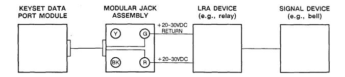
**NOTE:** Each time the keyset rings, the Data Port Module provides 20–26mA of loop current to the LRA. This causes the LRA contacts to close and activates the signalling device. The LRA is not affected by the ring tone or the ringer volume of the keyset. The LRA must be capable of operating on 20mA current (approximately 20VDC).
