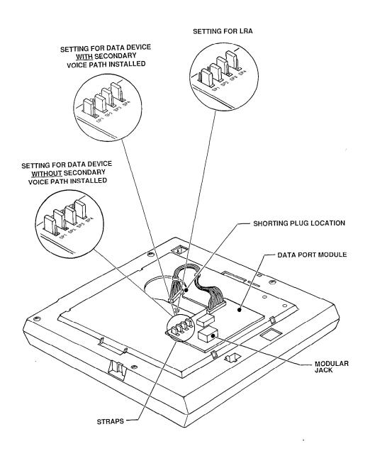
7.14 To Connect A Loud Ringing Adapter (LRA): The optional Data Port Module can be used to connect external signalling equipment such as loud bells, horns, flashing lights, etc. to a 24-line keyset. This application is useful in areas where the normal ring tone of the keyset cannot be heard, such as warehouses and loading docks. The signalling device follows the normal ringing patterns of the keyset.
