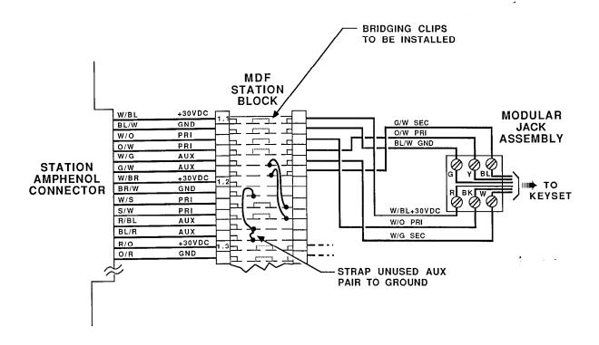
NOTE: For proper keyset operation, all three pairs (power/ground, primary, and secondary) are required.
