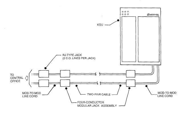
FIGURE 3-11. MODULAR JACK ASSEMBLY WIRING FOR C.O. LINES
