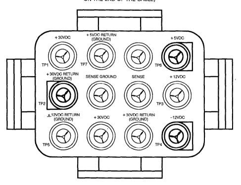
TP1 TO TP2 +30  $\pm 2.0$ VDC (+28VDC TO +32VDC)
