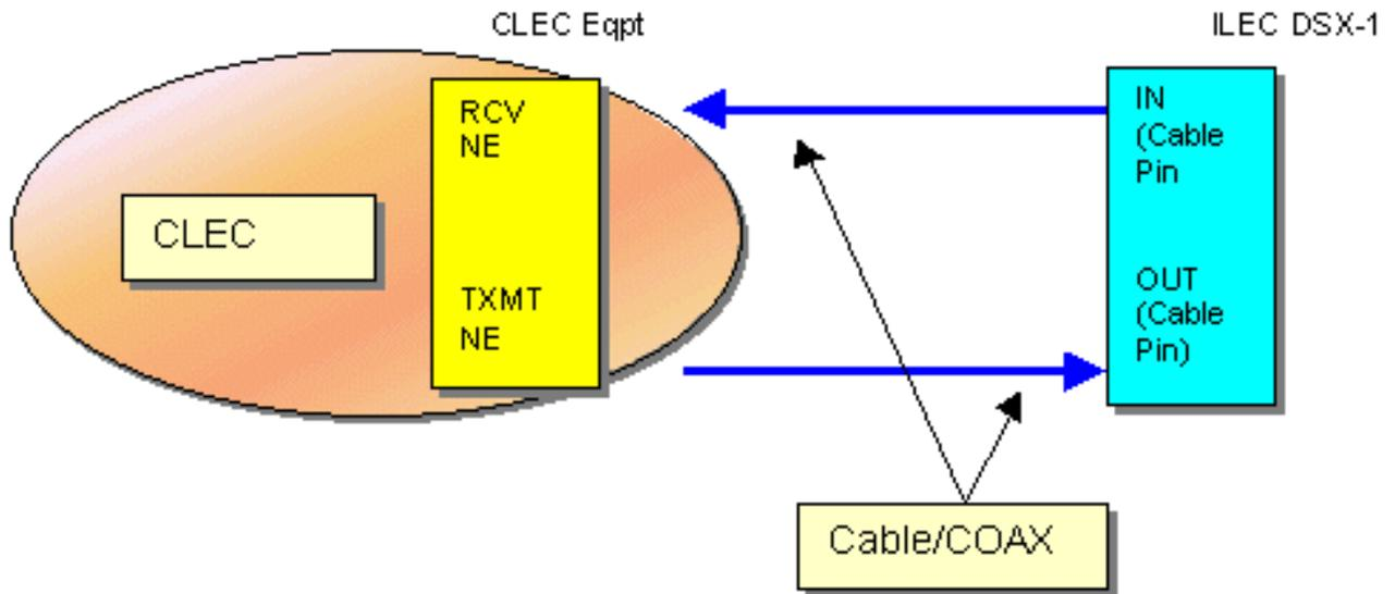
**C. ILEC Handoff to CLEC with CLEC Provided POT using one DSX**
