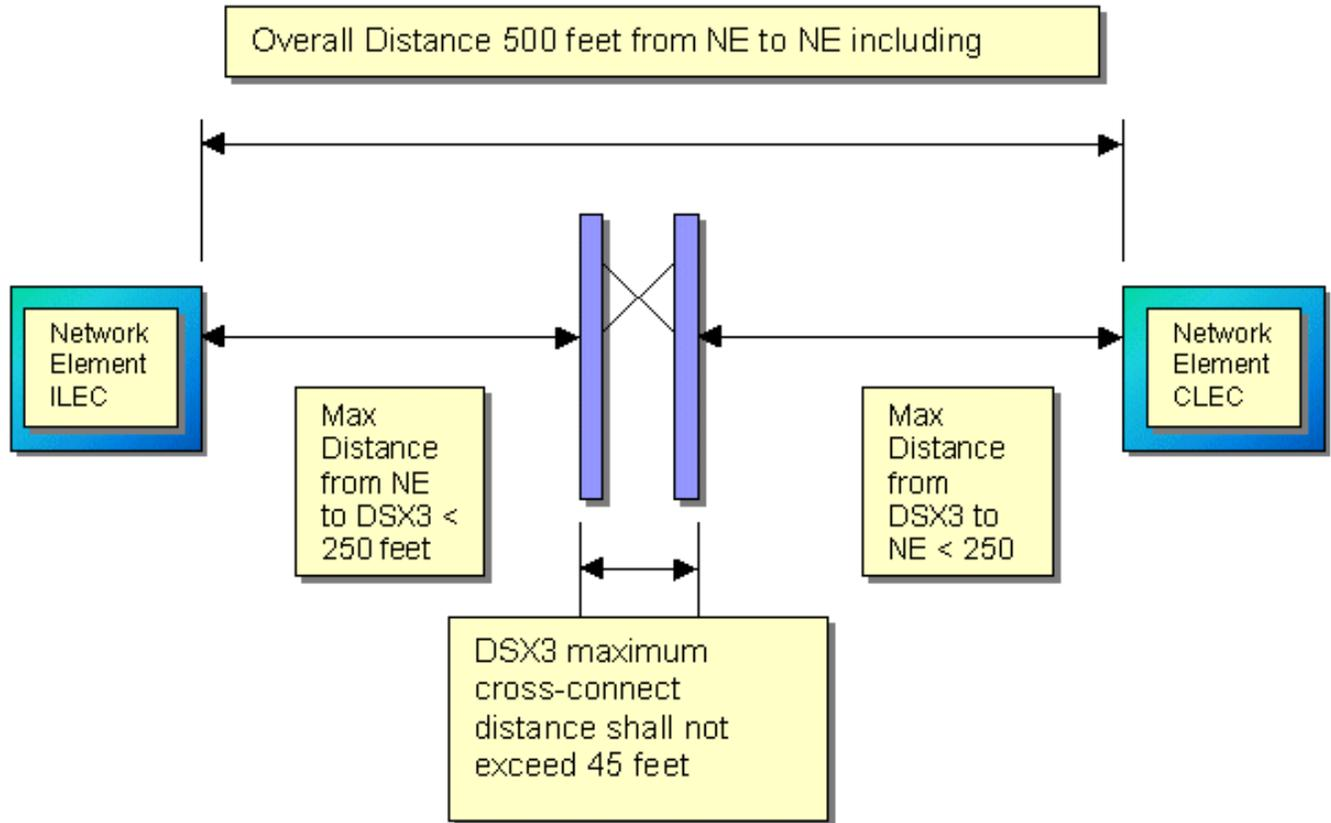
19. In cases where this distance limit cannot be met to the CLEC from ILEC equipment, intraoffice repeaters or terminations on Digital Cross-Connect Systems (DCS) may be needed to regenerate the signal to meet service parameters for the circuit.
