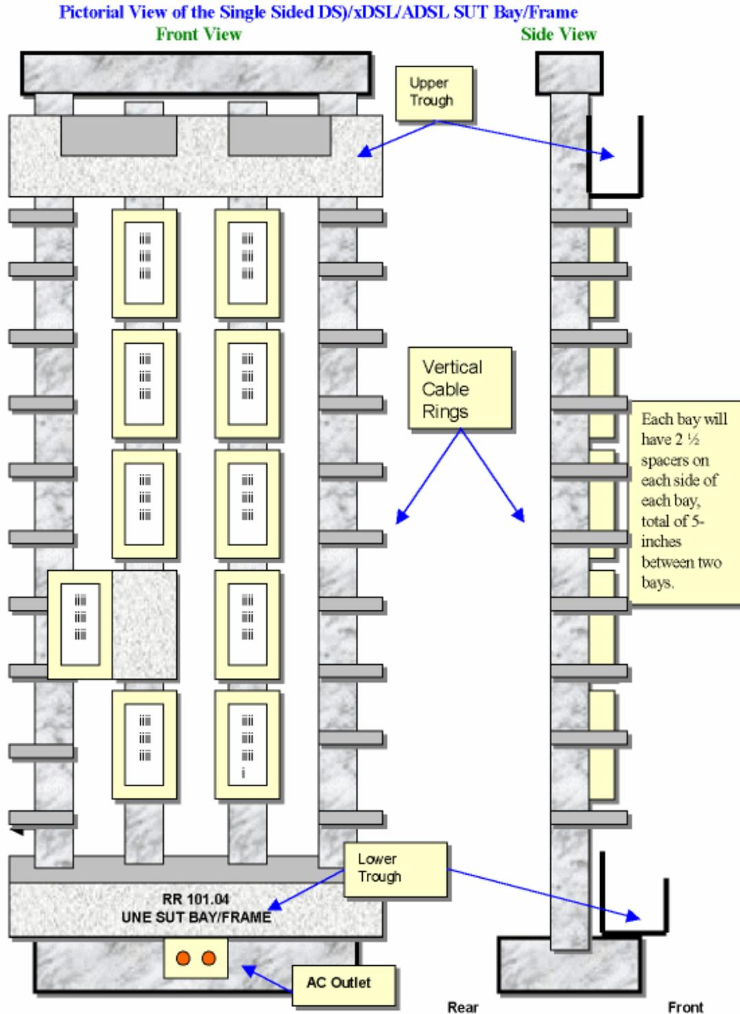
This illustration shows how a DS0 Collocation Bay/Frame is arranged. The equipment will fit within a standard bay footprint and may be placed in an existing Cageless Collocation Lineup.
