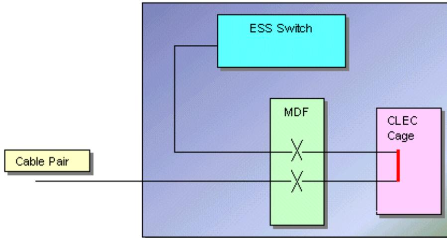
POTS Switch Port and Cable Pair connected using UNE Method 1 within the CLEC Physical Collocation Area. The CLEC connection is annotated in **RED**.
