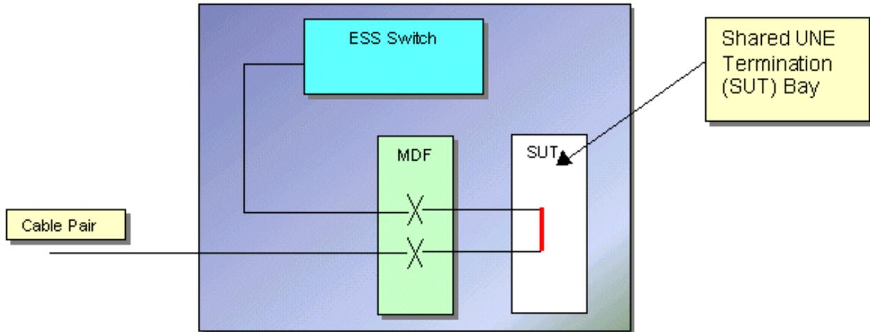
POTS Switch Port and Cable Pair connected using UNE Method 2 to a Shared UNE Termination Bay within the Collocation Area. The CLEC connection is annotated in **RED**.
