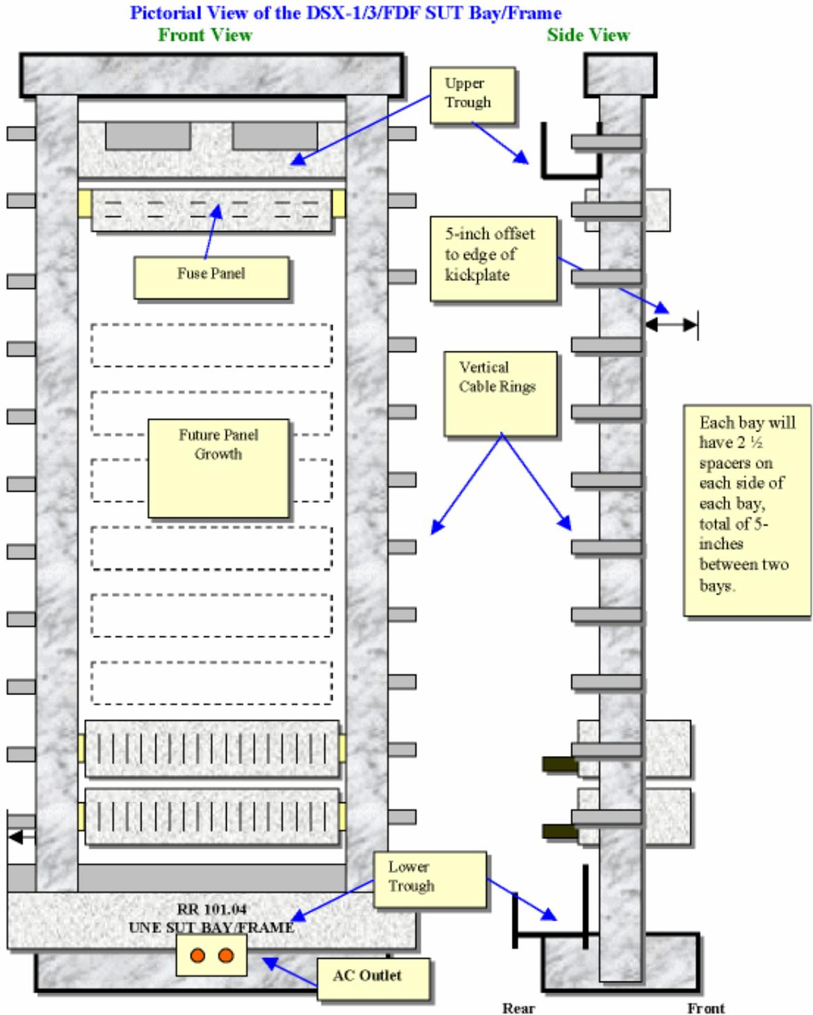
This illustration shows the typical layout of a standard DSX-1/3 or FDF Frame layout. Reference the standard SBC Drawings for the bay, troughs, rings and panels for deployment. The bay/frame will fit within an existing Cageless Collocation Lineup in a standard bay configuration.
