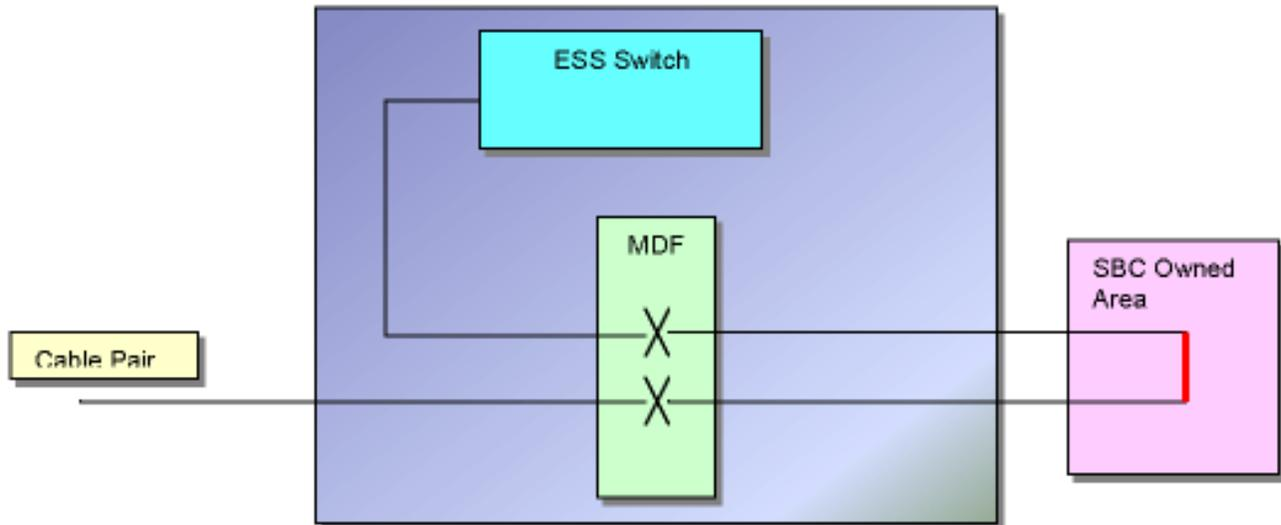
POTS Switch Port and Cable Pair connected using UNE Method 3 within SBC Owned Area outside of the Central Office. The CLEC connection is annotated in **RED**.
