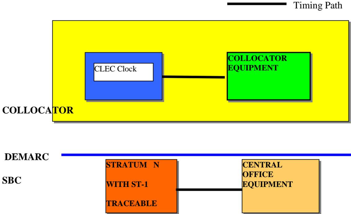
**18C. SBC Provisioned Timing using the BOR**
