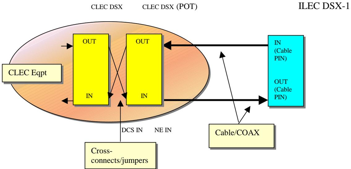
All Installation & Engineering workforces shall adhere to the following drawings for the correct termination of DDP (interconnect panels) with DSX panels in all Collocation activities. **Do not field modify these arrangements locally.**
