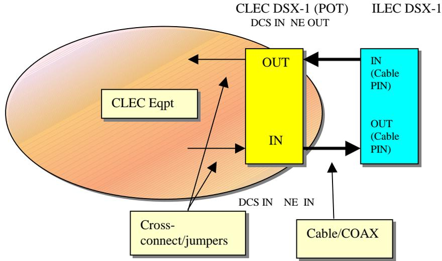
The CLEC needs to terminate their TMXT on the Cable PIN IN jack to the ILEC cable (to the ILEC OUT jack) and the Cable PIN OUT jack to the ILEC cable (to the ILEC IN jack). If the CLEC terminates in error to the cross-connect pins on their panel, they will have to change their cabling to match the ILEC or they will have to connect the services in a cross-connect manner (double cross) to compensate for the error. (The CLEC may be using a DDP with an internal reverse cross.)
