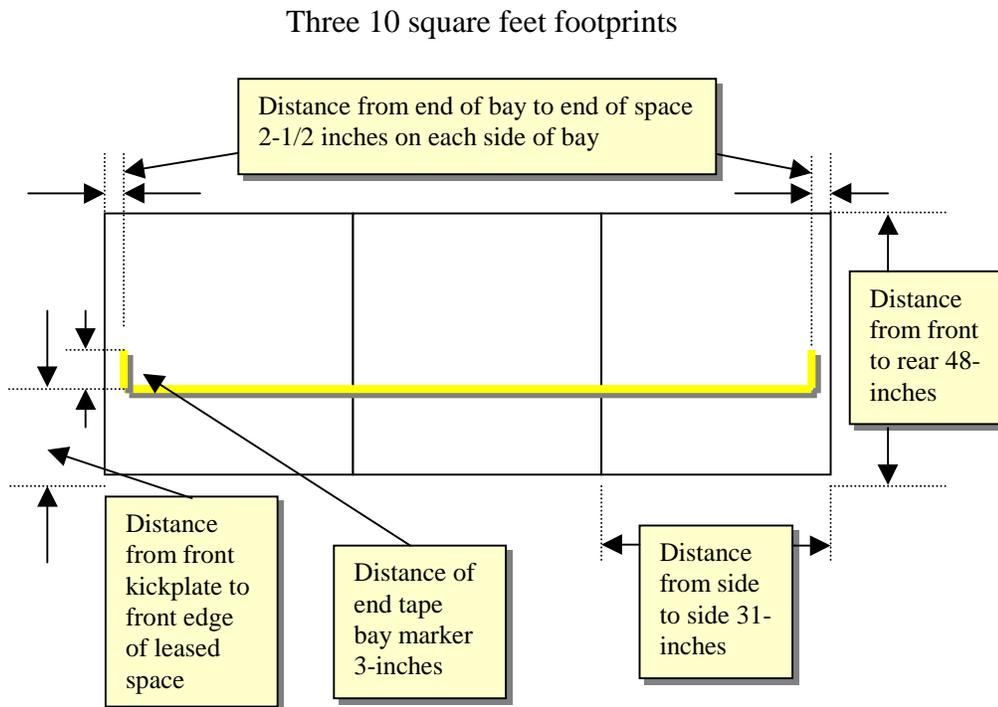
**Standard Bays footprint and floor marking with standard bay placement within each assigned area**
