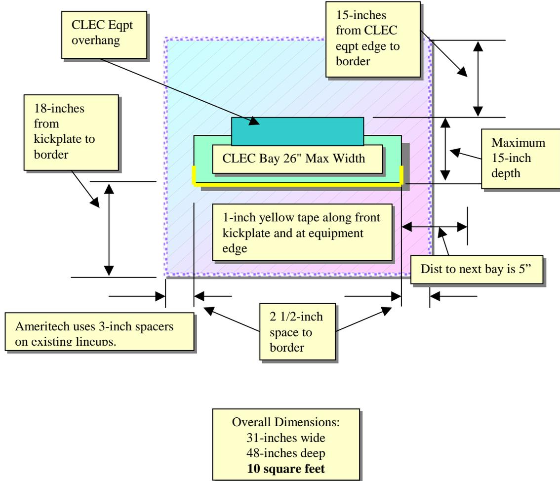
**Do not forget that for Collocation Installations the Standard Bay has a total of 36-inches from the front kickplate (tape) to the facing bay on the other side of the aisle. The rear to rear distance between bay and equipment should be no less than 2-ft 6-in.**
