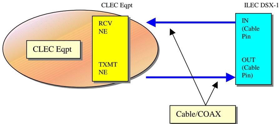
**C. ILEC Handoff to CLEC with CLEC Provided POT using one DSX**
