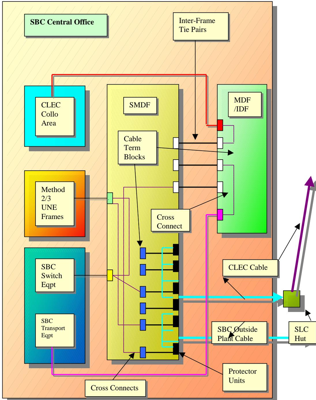
The illustration below provides a pictorial layout of a SBC Exchange Carrier cable and a CLEC cable Multiple Frame Central Office with a Universal Modular Distributing Frame
