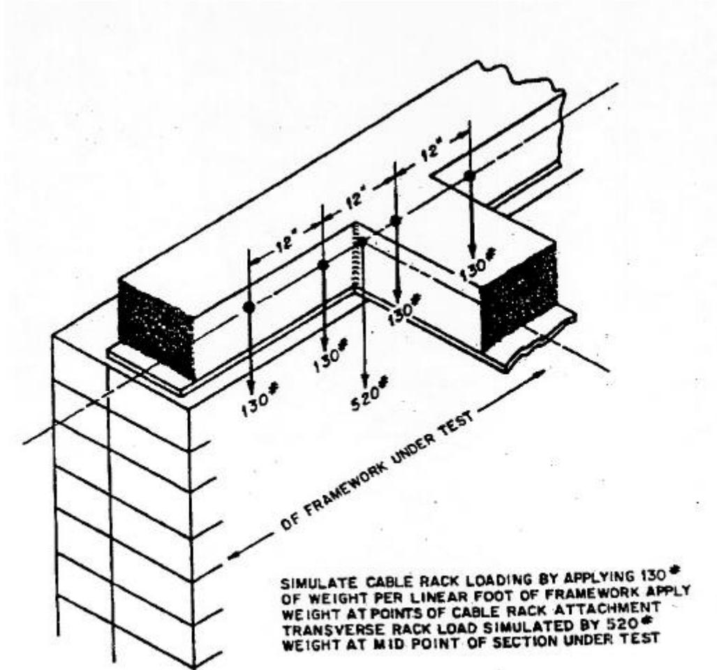
Figure 2. Apparatus Load – Horizontal
