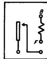
FIG. 8 - WINDING TERMINAL ARRANGEMENT AS VIEWED FROM THE FRONT (CONTACT SIDE) - 85 TYPE RELAY
