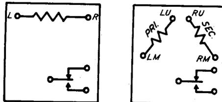
FIG. 13 - WINDING TERMINAL ARRANGEMENT AS VIEWED FROM THE REAR (TERMINAL SIDE) - 208 AND 214 TYPE RELAYS
