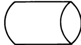
Fig. 20—Magnetic Drum Symbol
