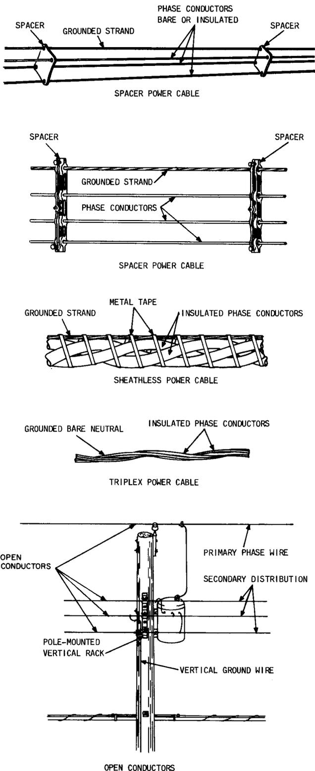
**Fig. 1—Types of Power Conductors**
