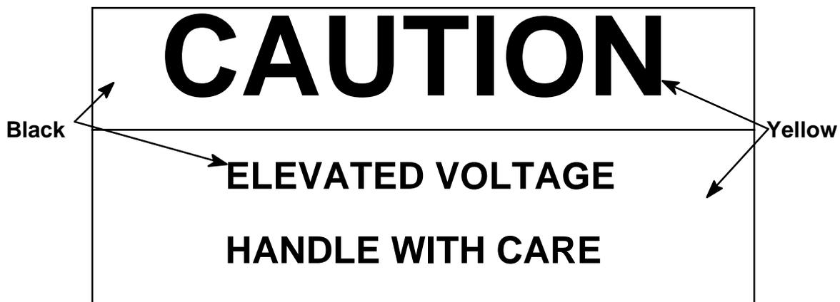
**Figure 1 - Typical Elevated Voltage Label**
