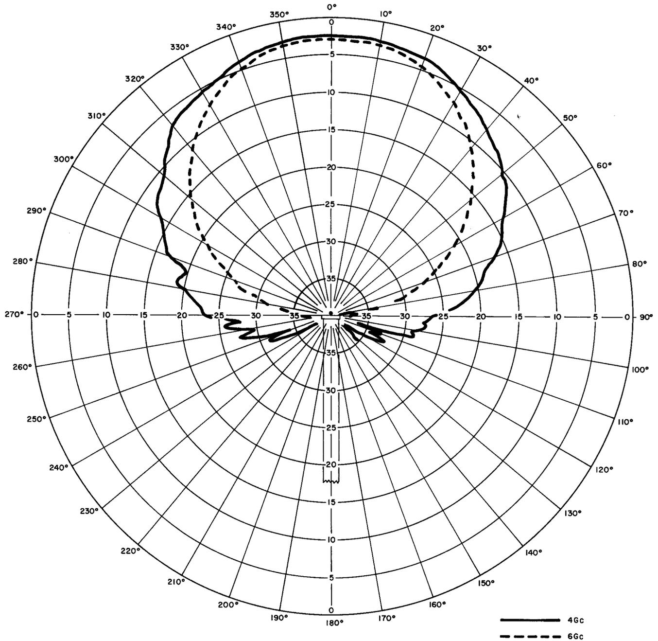
Fig. 2—Vertical Polarization Round Guide, H Plane
