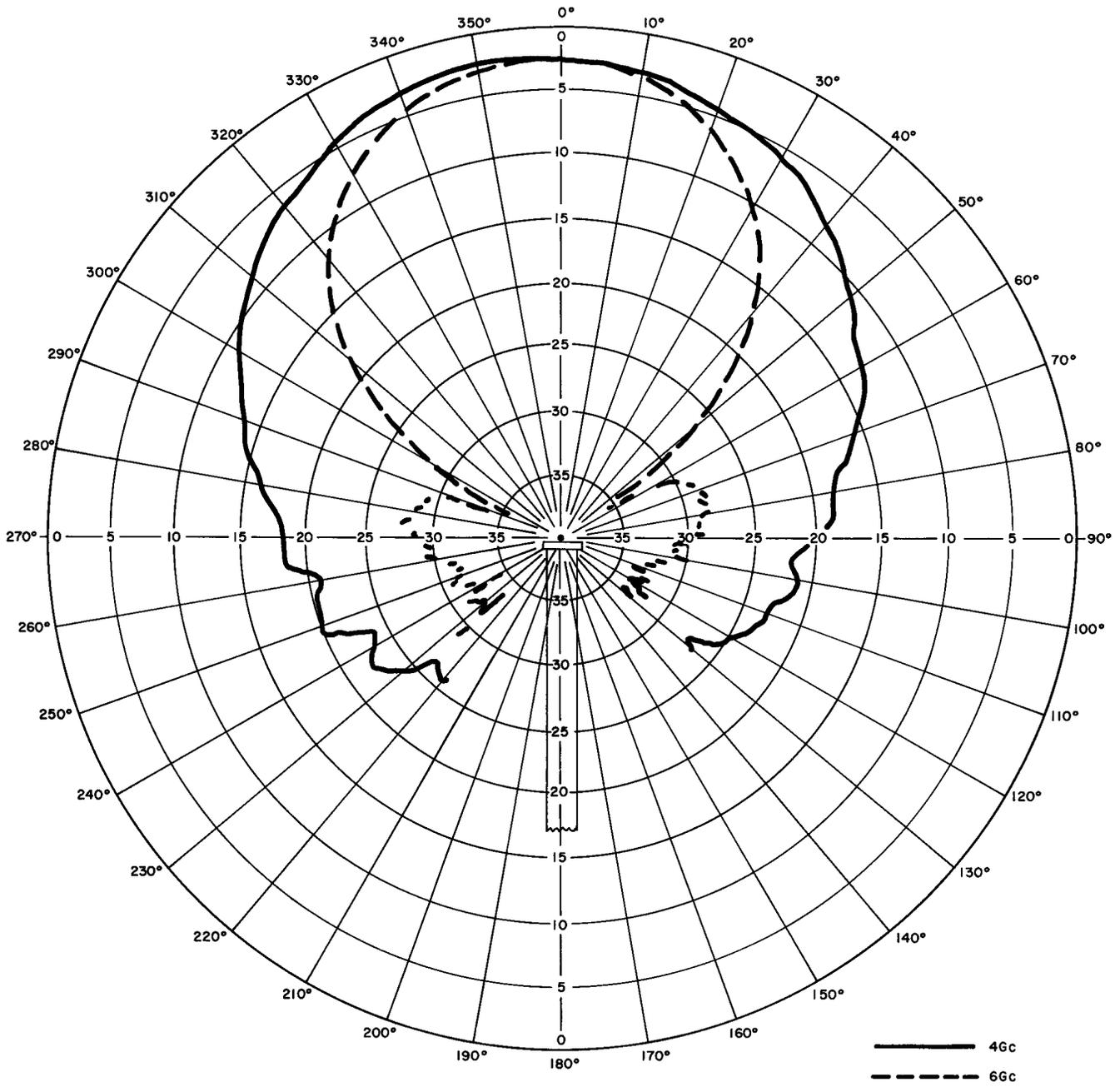
Fig. 3—Horizontal Polarization Round Guide, E Plane
