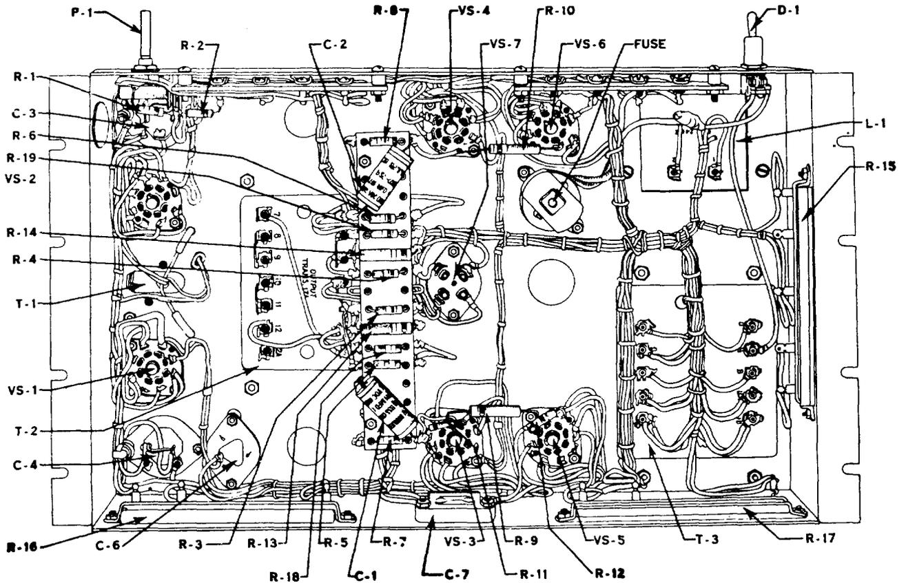
Fig. 3 - Bottom View of 118A Amplifier
