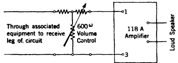
Fig. 7 - Station Circuits with Loud-speaker Signaling
