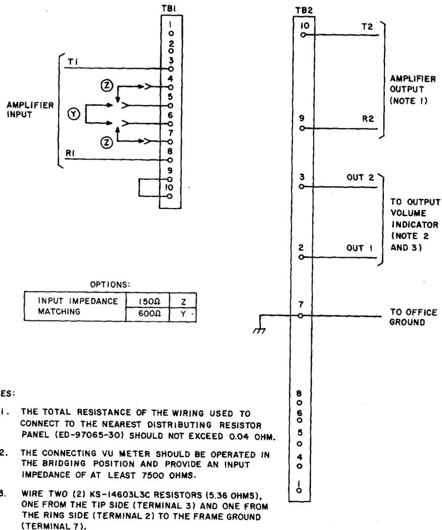
Fig. 1—KS-20425 L1 (Manufacture Discontinued) Amplifier System—Connections and Options
