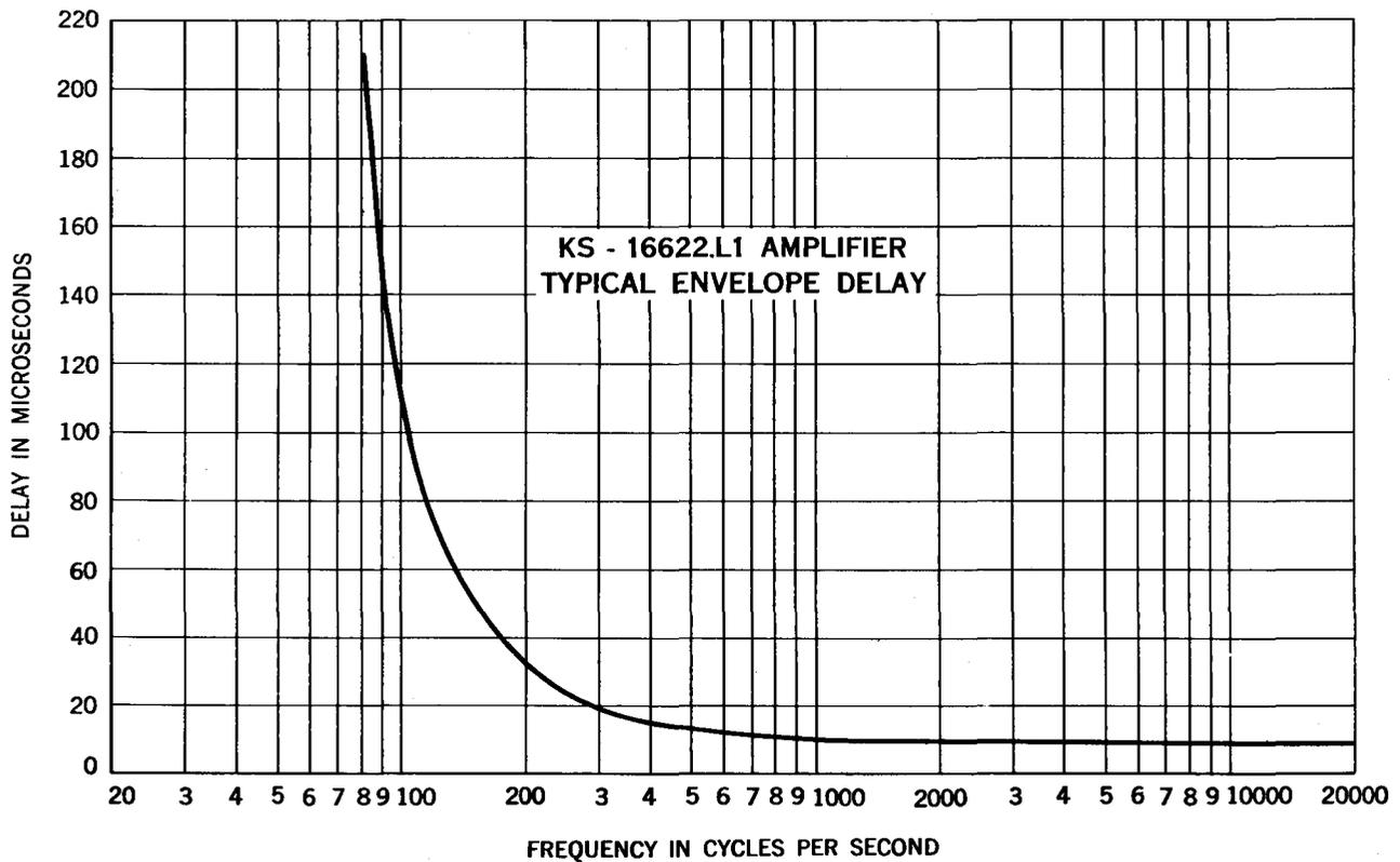
Fig. 6 - Envelope Delay Distortion
