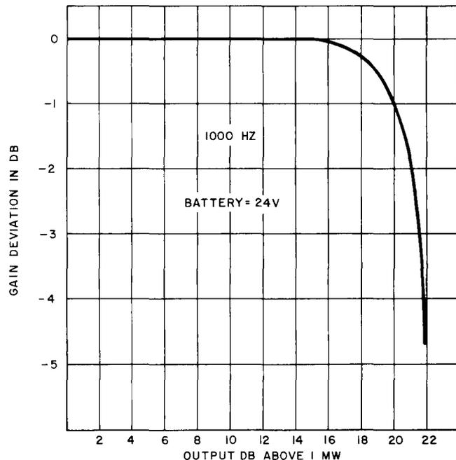
Fig. 10—227C or D Amplifier—Typical Output Load Carrying Capacity
