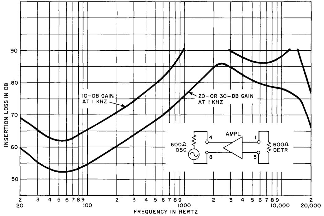
Fig. 11—227C or D Amplifier—Reverse Transmission Loss
