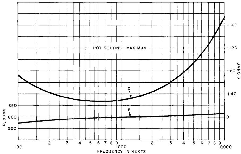
Fig. 4—227C or D Amplifier—Input Impedance—600-Ohm Termination
