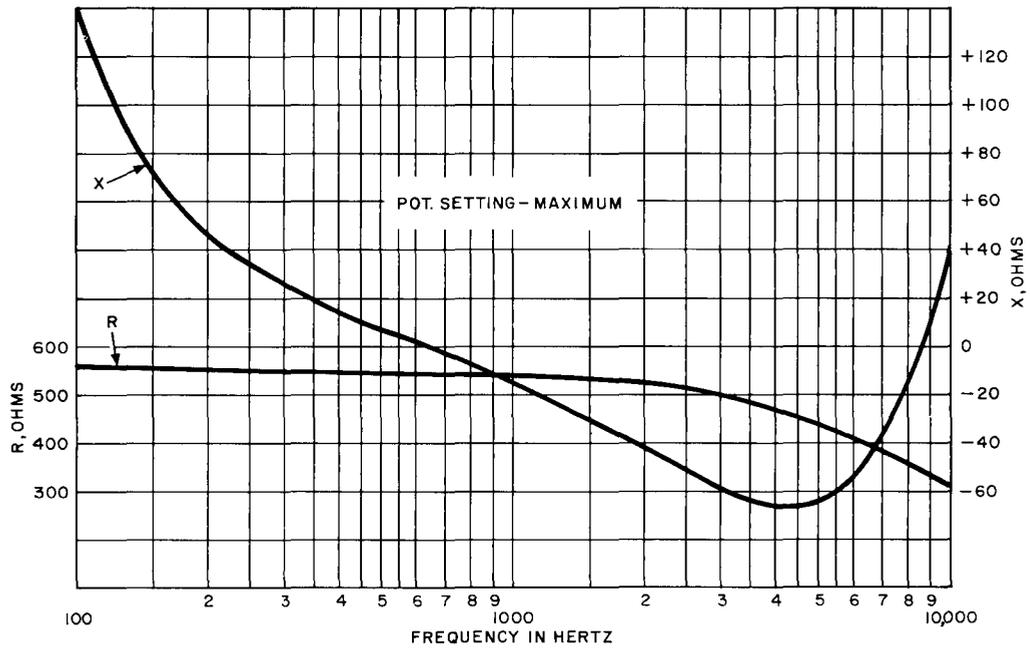
Fig. 5—227C or D Amplifier—Output Impedance—600-Ohm Termination
