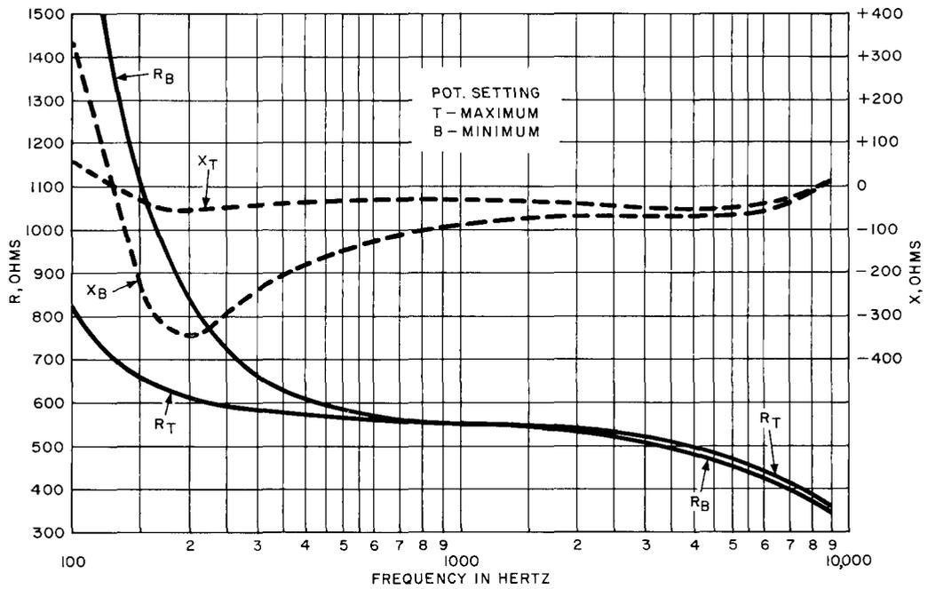
Fig. 6—227C or D Amplifier—Output Impedance—600-Ohm Termination
