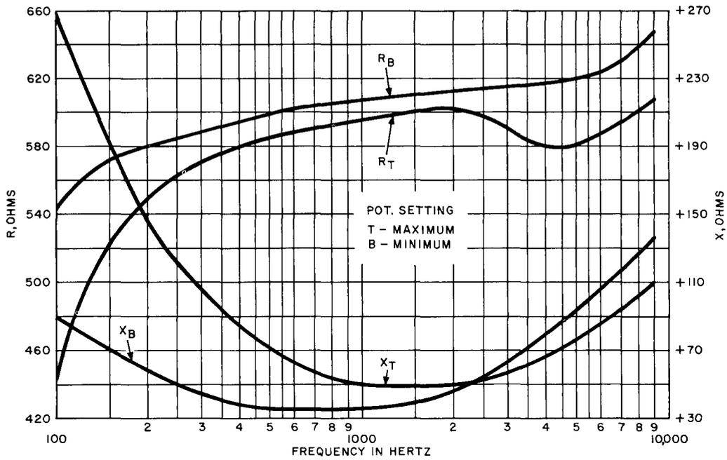
Fig. 3—227C or D Amplifier—Input Impedance—600-Ohm Termination
