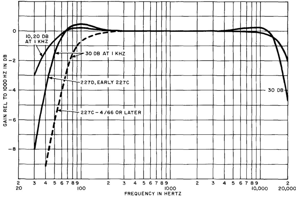
Fig. 7—227C and D Amplifiers—Gain-Frequency Characteristics
