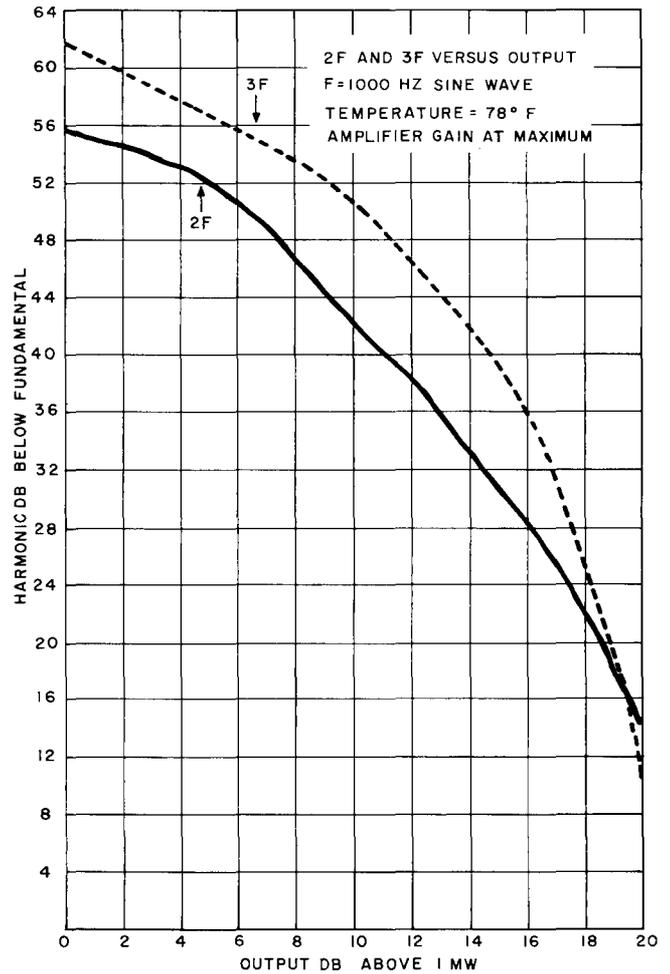
Fig. 9—Harmonic Content of 227C Amplifier (4/66 or Later Production)
