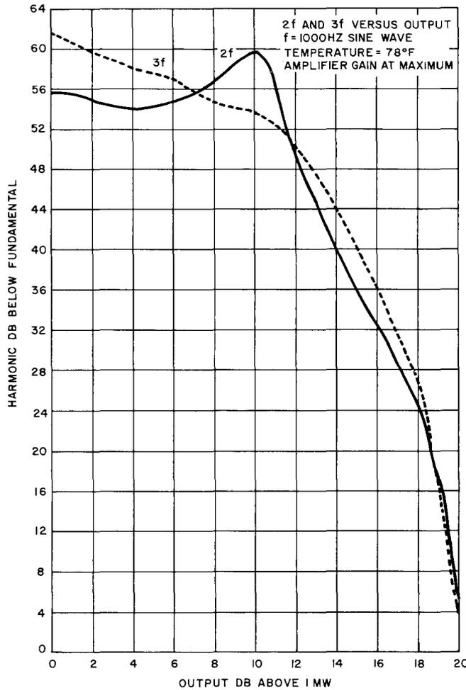
Fig. 8—Harmonic Content of 227C Amplifier (3/66 or Earlier Production) and 227D Amplifier
