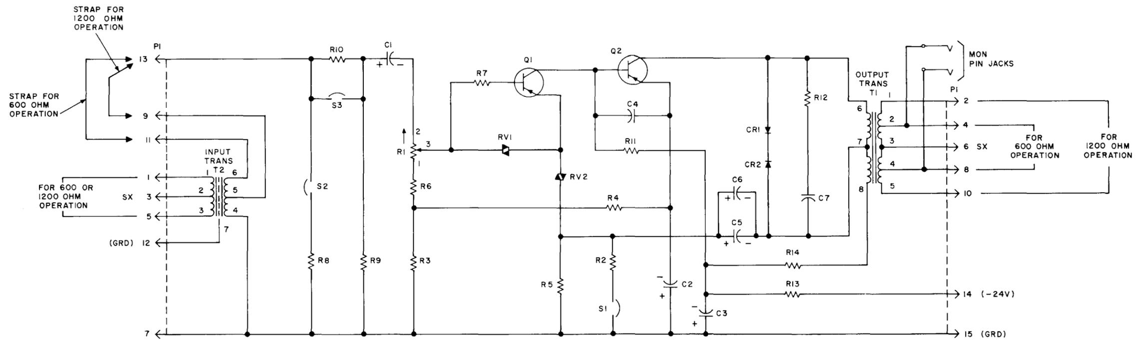
Fig. 2—227C or D Amplifier—Schematic and Faceplate Arrangement
