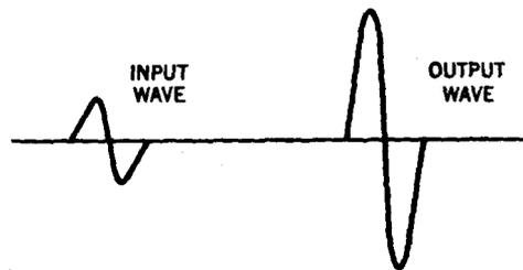
Fig. 8—Comparison of Input and Output Waveshapes (Distortion)
