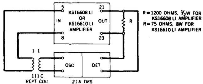
**Fig. 1—Test Setup for Gain-Frequency Test—High Impedance Input**
