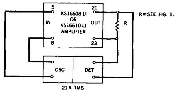
**Fig. 2—Test Setup for Gain-Frequency Test—Transformer Input**
