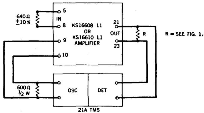
**Fig. 5—Test Setup for Gain-Frequency Test—Bridging Input**
