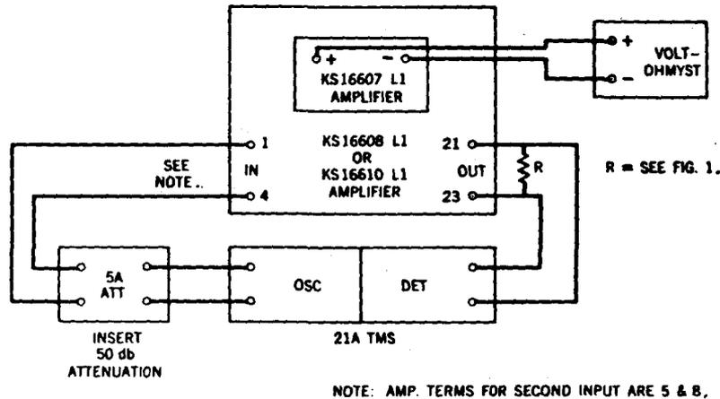
Fig. 9—Test Setup for Limiter Test
