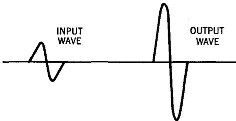
Fig. 4 - Comparison of Input and Output Waveshape (Distortion)
