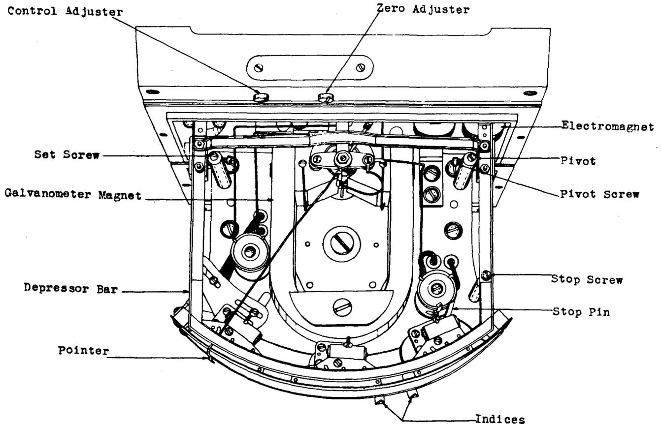
Fig. 7 Top View of Controller
