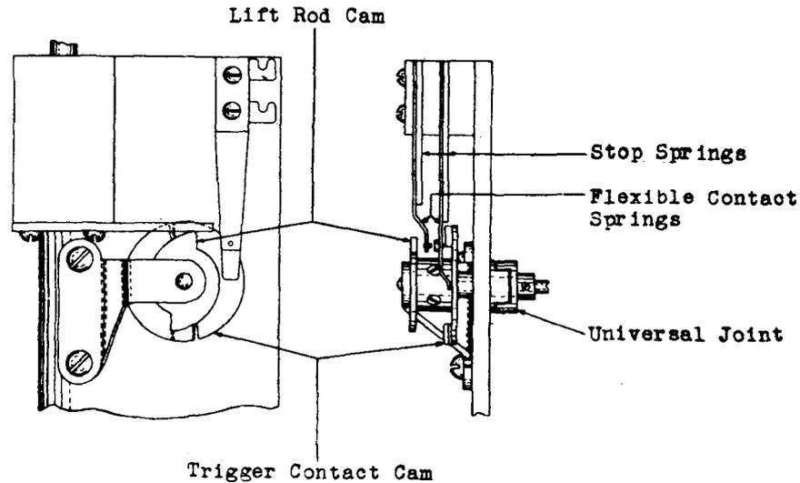
Fig. 11 Trigger Contact - Direct Cam Type
