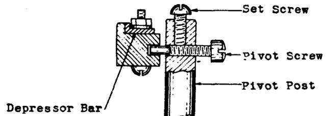
Fig. 9 Depressor Bar Pivot
