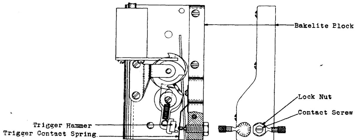
Fig. 6 Trigger Contact - Hammer Type
