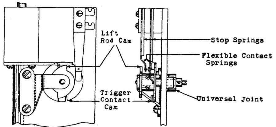
Fig. 5 Trigger Contact - Direct Cam Type
