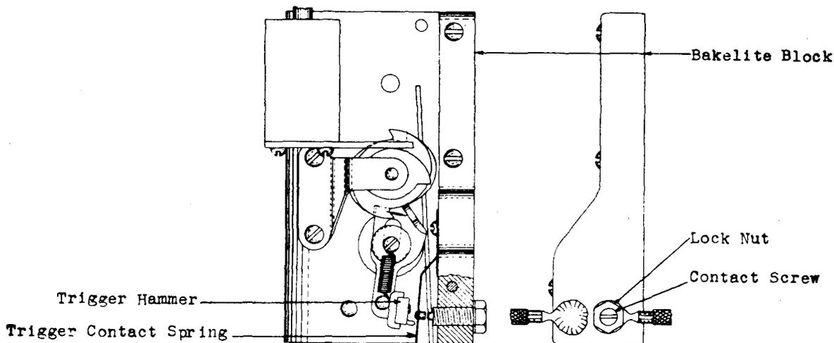
Fig. 12 Trigger Contact - Hammer Type
