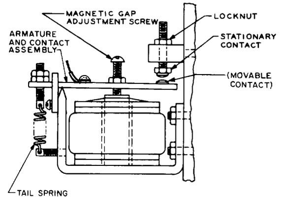
Fig. 8—Series Relay (part of KS-5755 starter shown)
