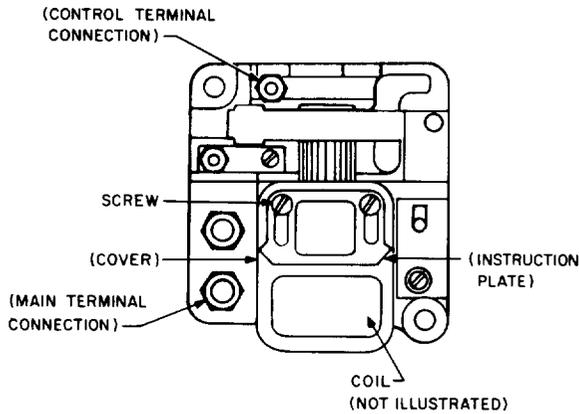
Fig. 5—Overload Relay (part of KS-5755 starter shown)
