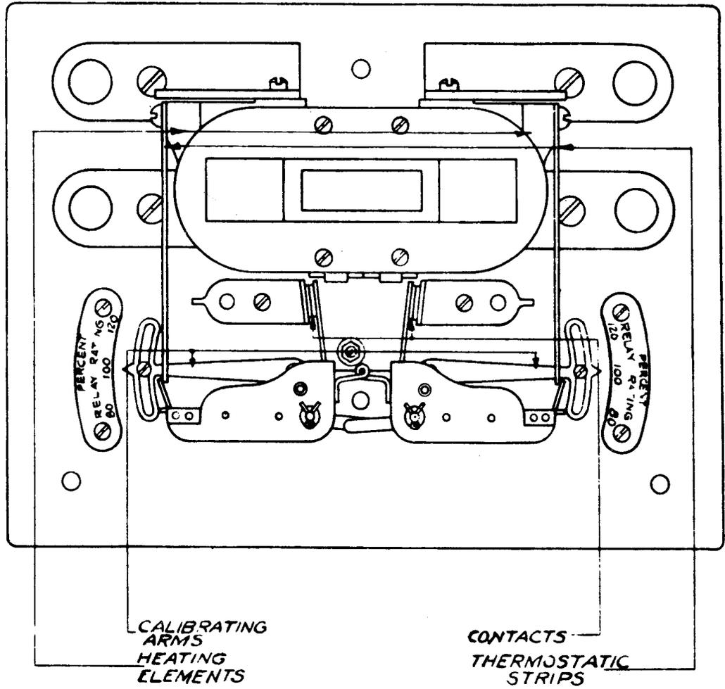
Fig. 3 - Hand Starting Compensators For Polyphase Motors-Temperature Overload Relay
