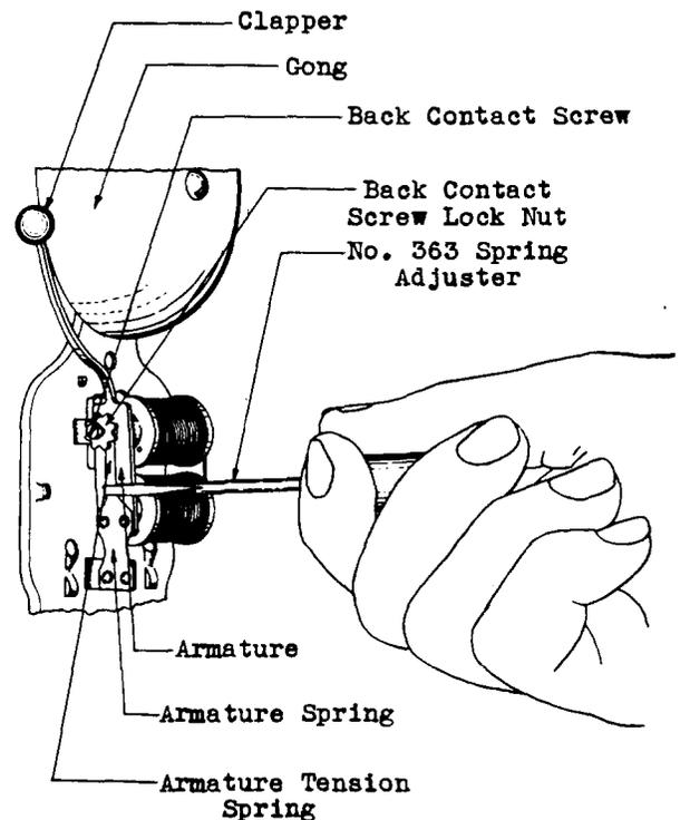
Fig. 4 - Method of Tensioning Armature Tension Spring
