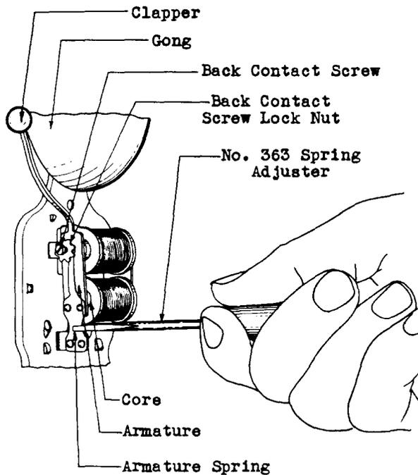
Fig. 3 - Method of Tensioning Armature Spring
