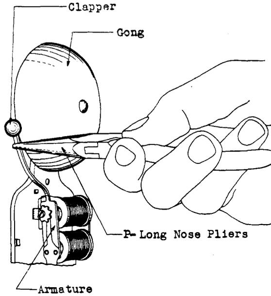
Fig. 5 - Method of Adjusting for Clapper Movement
