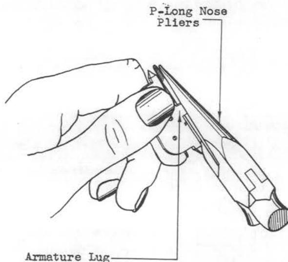
Fig. 3 - Method of Adjusting Armature Lug Nos. 2-D and 2-E Buzzers
