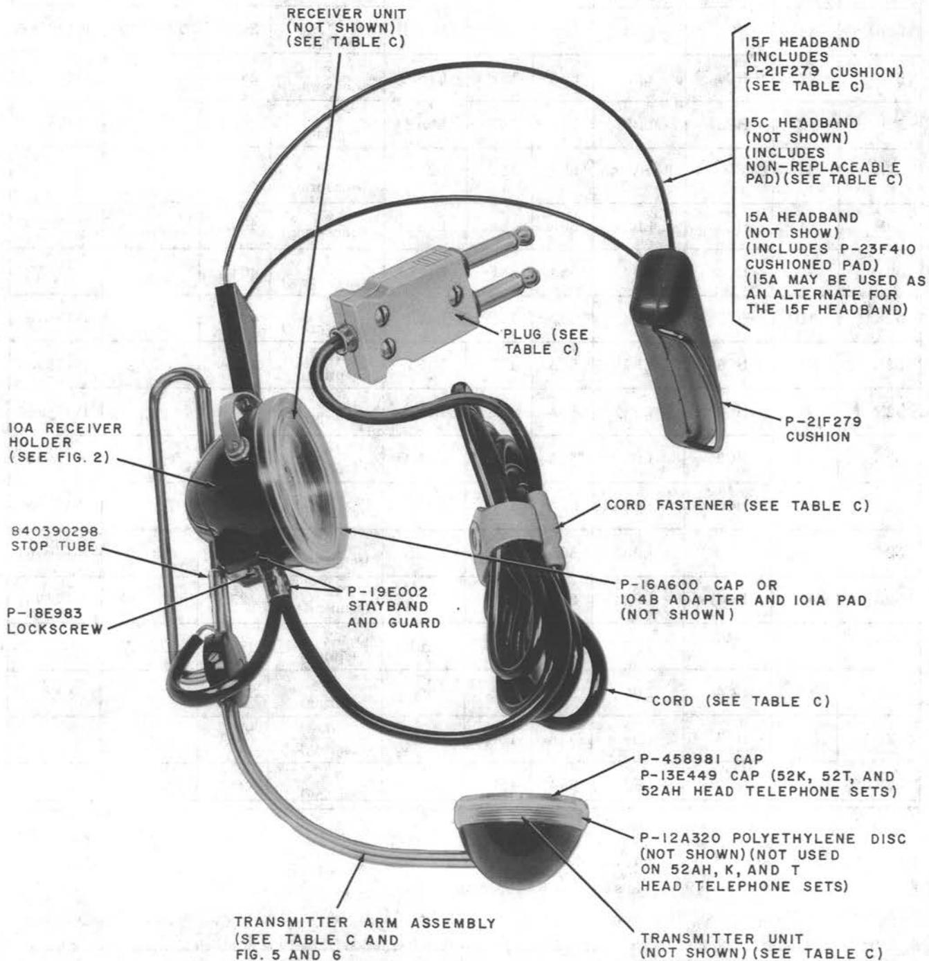
Fig. 1—52-Type Head Telephone Sets (52S Head Telephone Set Equipped With Stopbar Illustrated)
