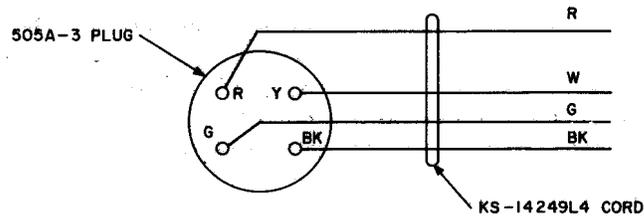
Fig. 10— 505A-3 Plug Connections
