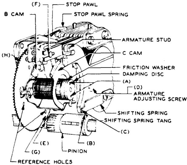
Fig. 5 - Engagement of Shifting Spring Tang and Pinion
