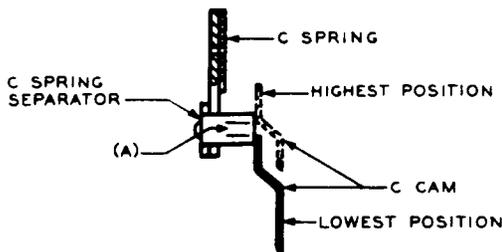
Fig. 17 - "C" Cam Position (Front View)
