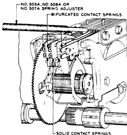
Fig. 23 - Method of Adjusting Spring Tension
