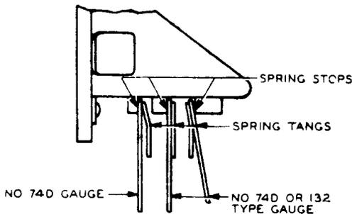
Fig. 13 - Method of Gauging Contact Springs
