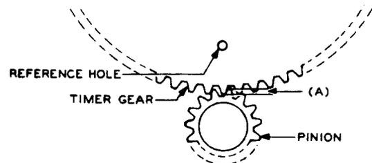
Fig. 4 - Engagement of Timer Gear and Pinion
