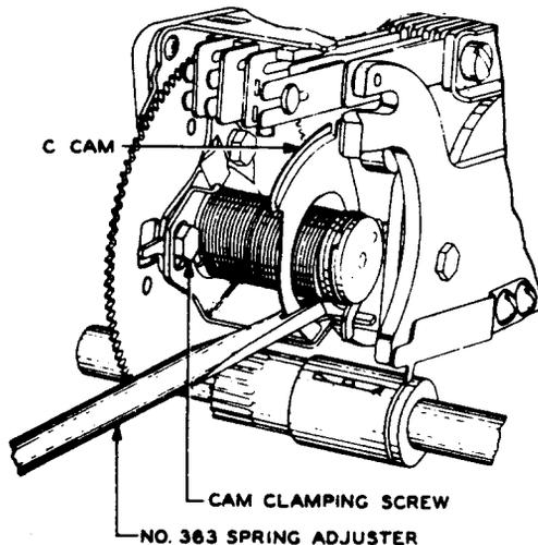
Fig. 26 - Method of Adjusting "C" Cam
