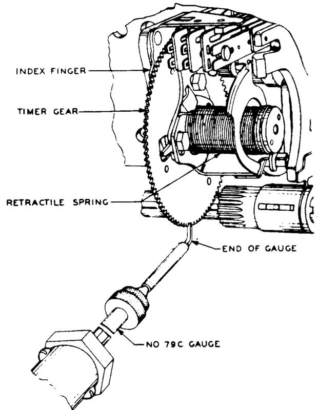
Fig. 18 - Checking Retractable Spring Tension
