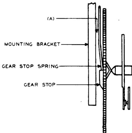
Fig. 10 - Gear Stop Spring Position
