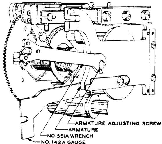
Fig. 21 - Method of Adjusting Armature Travel
