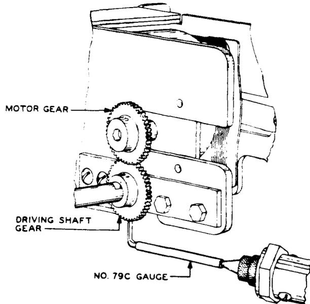
Fig. 6 - Method of Checking Freedom of Shaft Movement
