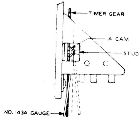
Fig. 15 - Checking "A" Cam Position
