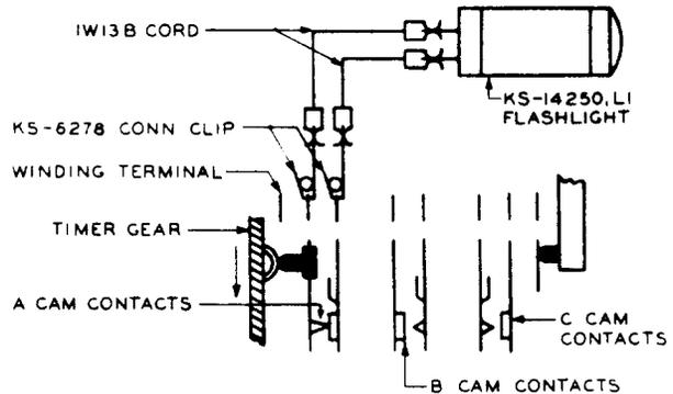
**Fig. 20 - Connections for Checking Timing Interval**
