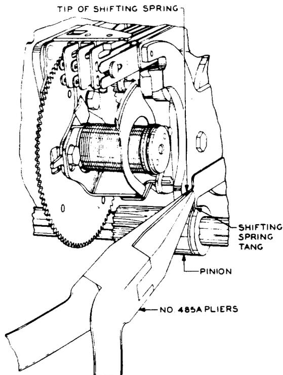
Fig. 22 - Method of Adjusting Shifting Spring
