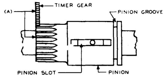
Fig. 8 - Engagement of Pinion With Associated Gear
