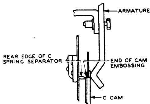
Fig. 25 - Method of Adjusting "C" Cam
