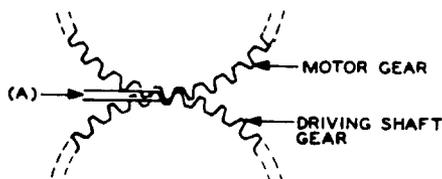
Fig. 3 - Engagement of Motor and Driving Shaft Gears
