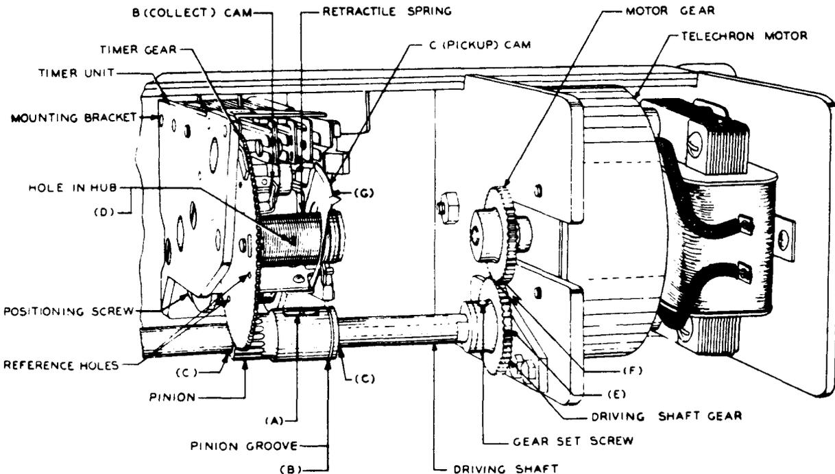
Fig. 2 - Timer and Associated Drive Assembly
