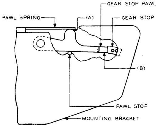
Fig. 9 - Gear Stop Pawl Position
