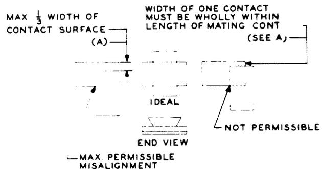
L Fig. 12 - Alignment of Heavy Contacts
