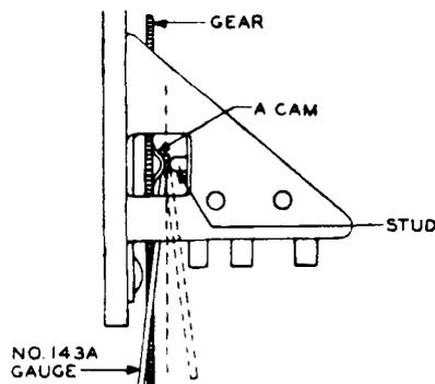
Fig. 24 - Method of Adjusting "A" Cam
