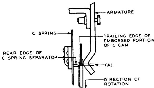
Fig. 16 - "C" Cam Position (Top View)
