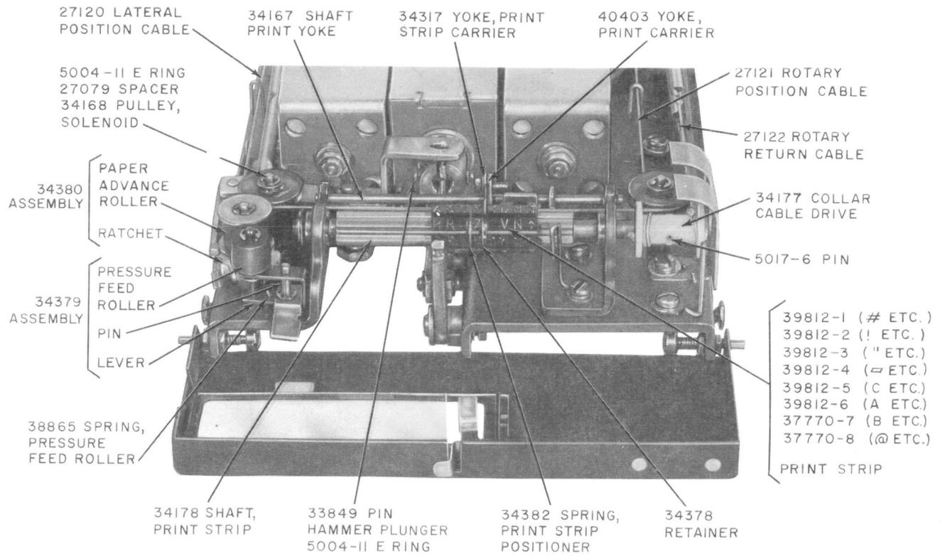
Fig. 2—KS-19717 L6 Tape Printer Showing Print Segments
