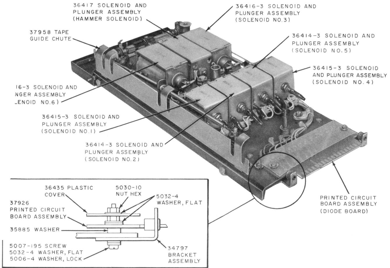
**Fig. 3—KS-19717 L6 Tape Printer Showing Circuit Board**
