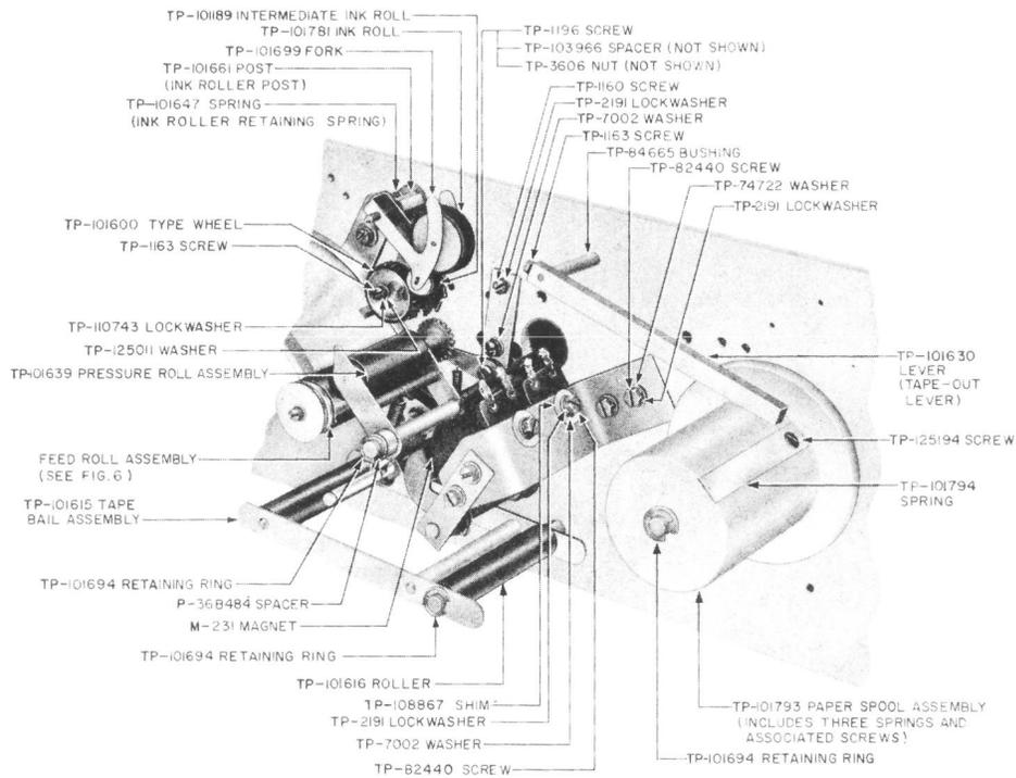
Fig. 5—Printing Mechanism (top view)
