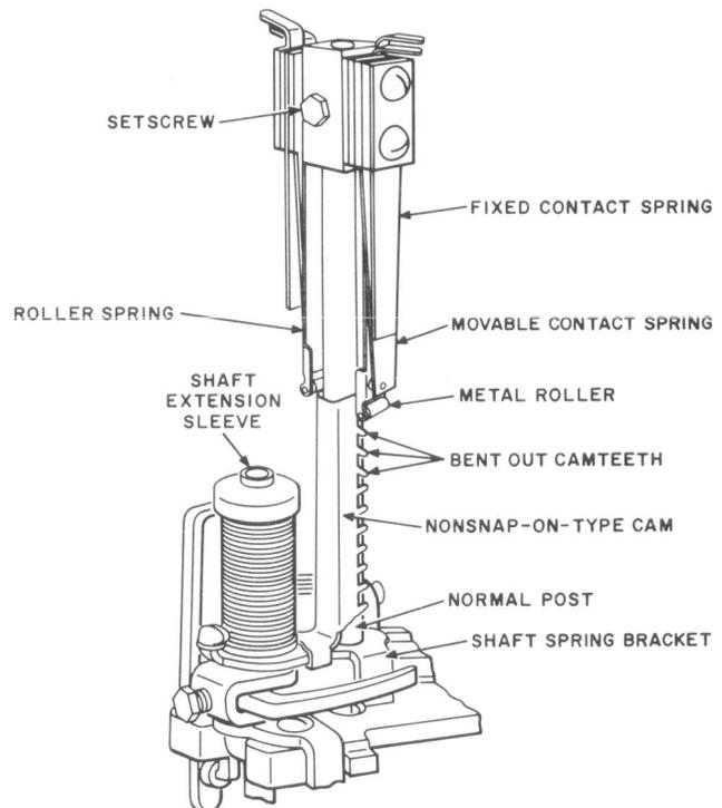
Fig. 14—Normal Post Spring Assembly Having Metal Rollers Operated by Nonsnap-on-Type Cam
