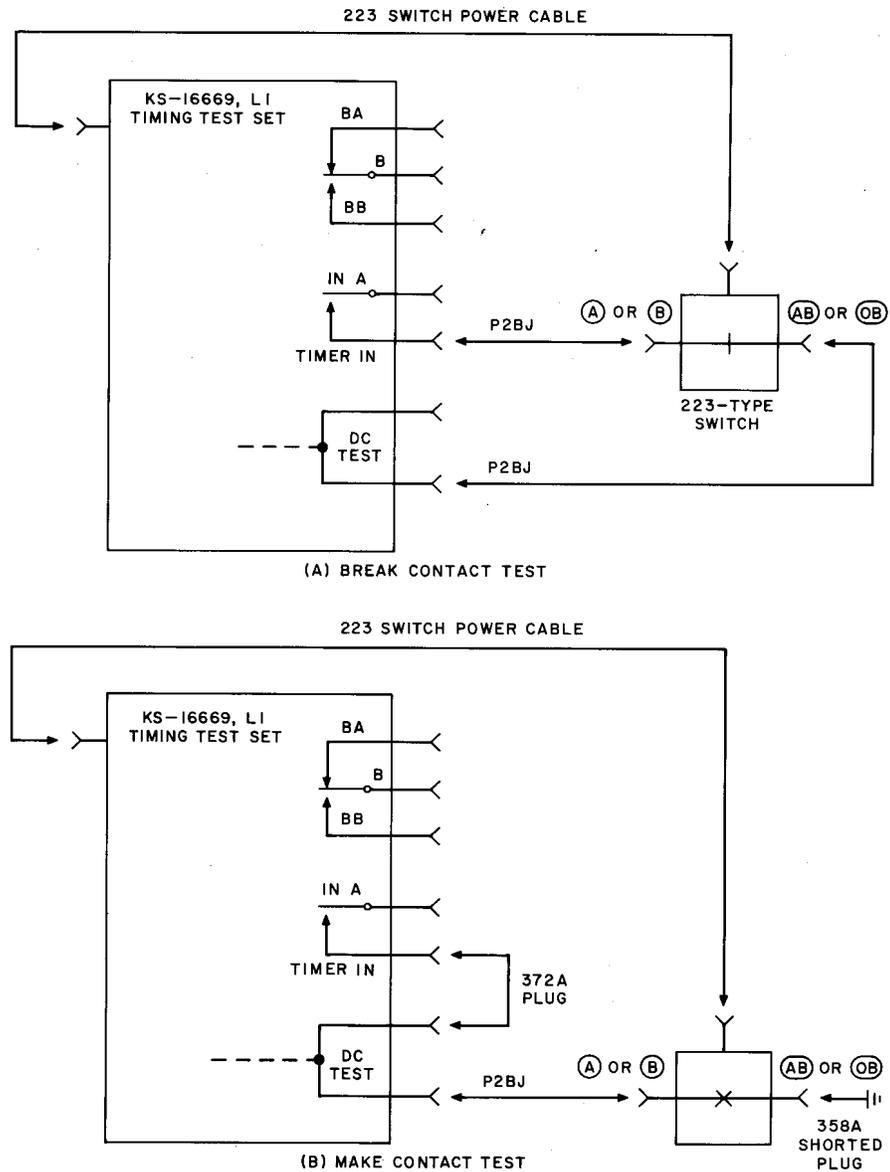
Fig. 16—Test Arrangement for 223-Type Switch Timing Tests
