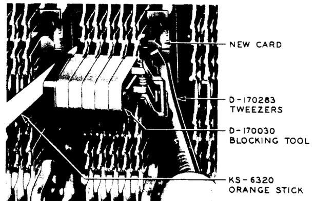
Fig. 10 - Final Positioning Operations of New Card
