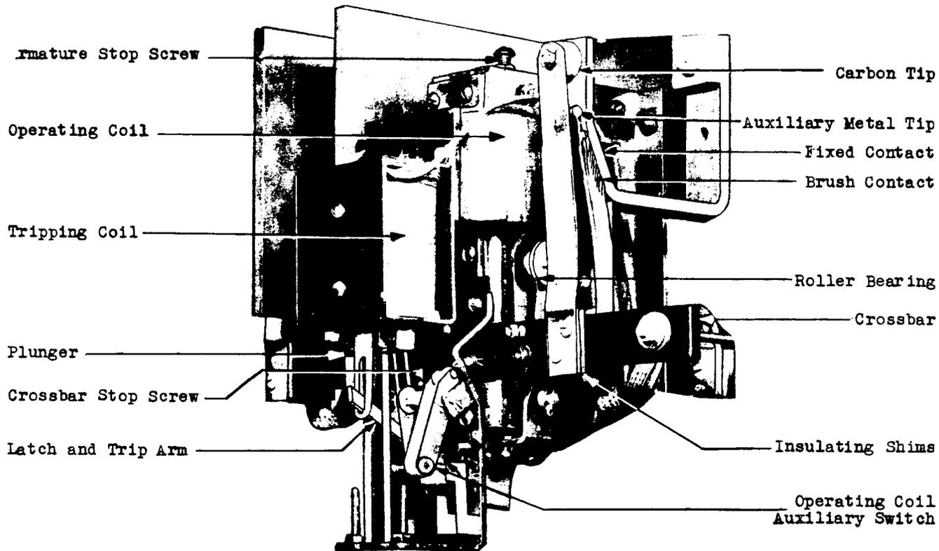
Fig. 5 - Contactor, Trip and Latch Mechanism
