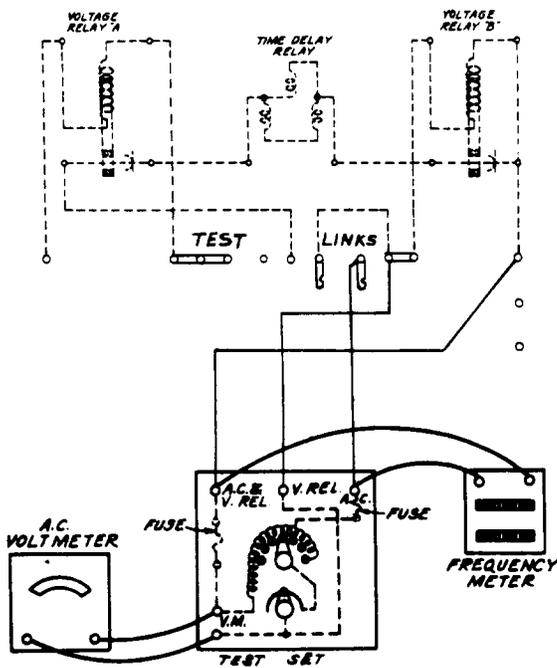
Fig. 7 - Test Connections for Relay "B" Without Transformer
