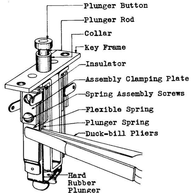
Fig. 6 - Method of Adjusting Contact Springs
