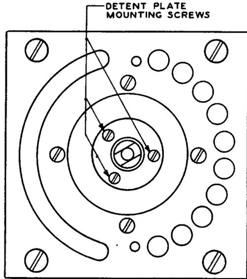
KNOB AND SPRING ASSEMBLY REMOVED
