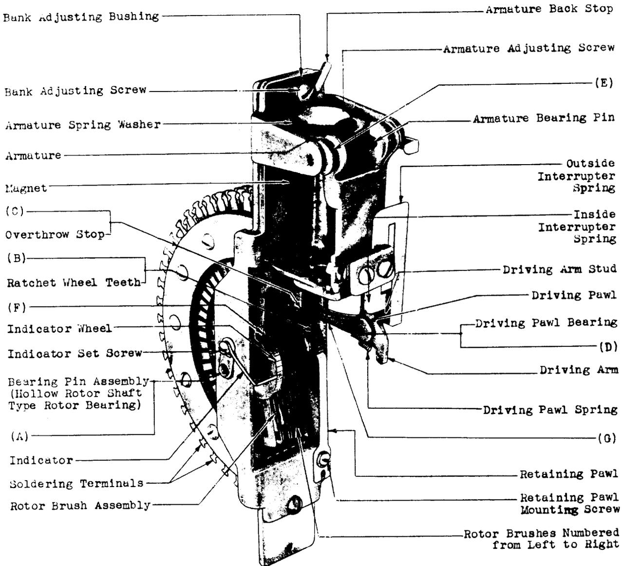
Fig. 1 - Heavy-Duty, 25-Point Rotary Switch
