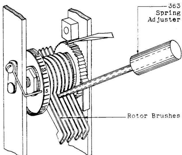
Fig. 9 - Method of Adjusting for Brush Alignment
