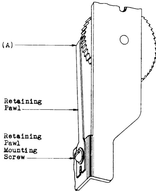
Fig. 5 - Position of Retaining Pawl Spring
