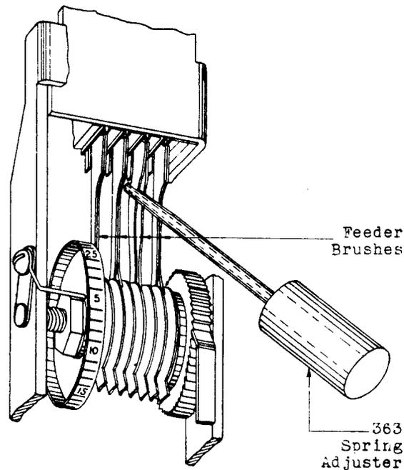
Fig. 8 - Method of Adjusting for Feeder Brush Closure
