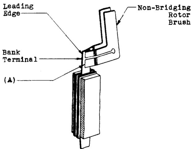
Fig. 4 — Position of Nonbridging Rotor Brush on Bank Terminal
