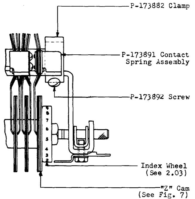
Fig. 9 - "Z" Cam Spring Assembly and Mounting Clamp
