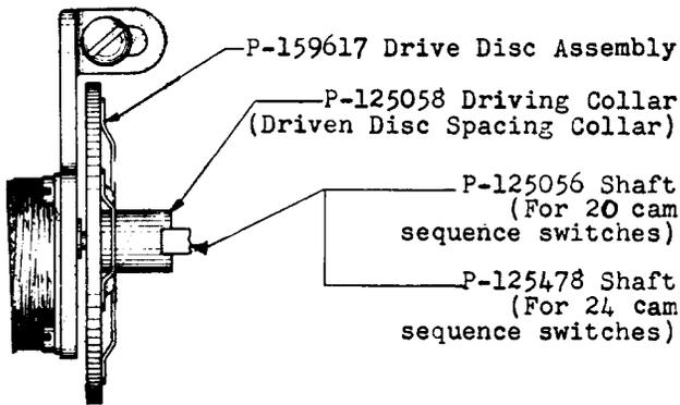
Fig. 3 - Driven Disc and Associated Parts
