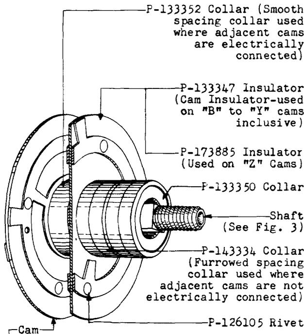
Order cam by the letter indicating its position and give the code number of the sequence switch. For example: "C" cam for the A231 sequence switch. (See 3.31) If a contact plate blank (without cutting) is desired, order P-173779 contact plate blank (silver overlay).
