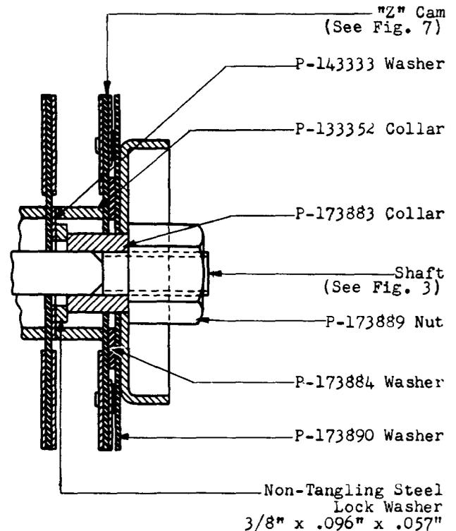
Fig. 10 - "Z" Cam and Associated Parts
