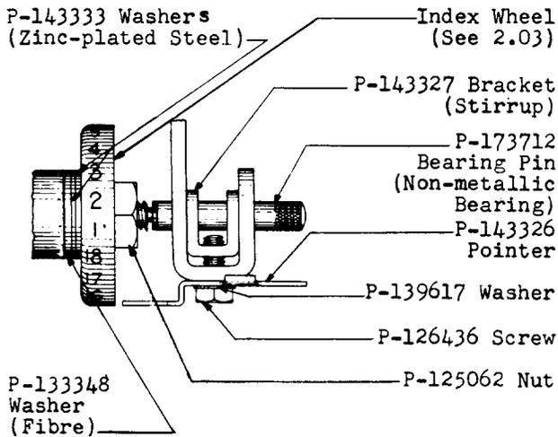
Fig. 2 - Bearing Pin and Associated Parts
