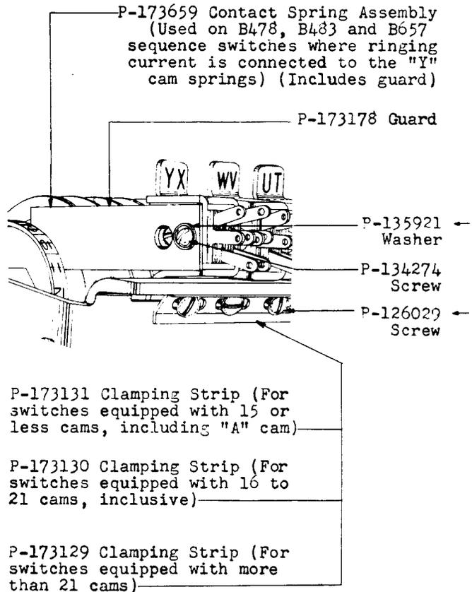
Fig. 6 - Clamping Strip and "Y" Cam Guard
