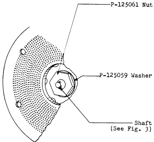
Fig. 5 - Driven Disc Clamping Nut and Washer
