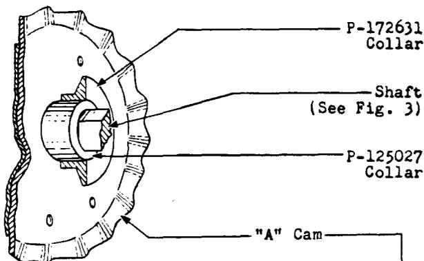
When ordering a new "A" cam indicate the code No. of the sequence switch on which it is to be used.
