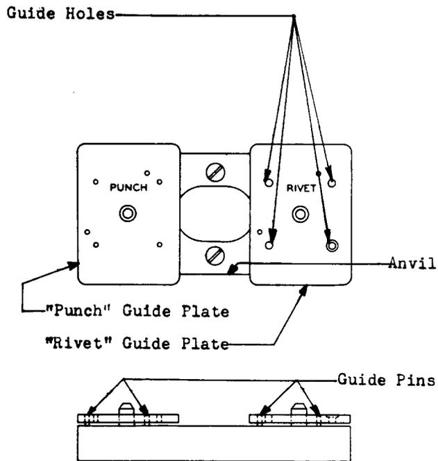
Fig. 23 - No. 397A Anvil and Guide Plates
