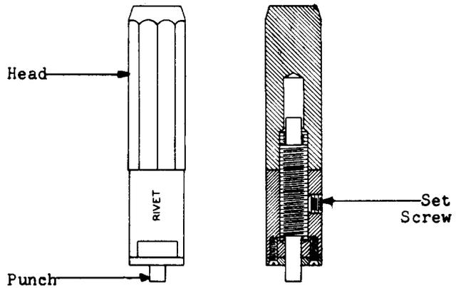
Fig. 22 - No. 398B Rivet Heading Punch
