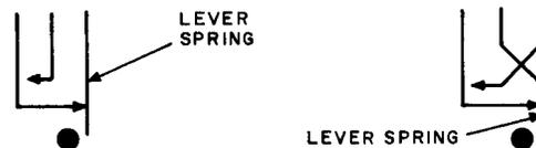
**Fig. B—Special Make-Before-Break Contact Springs**
