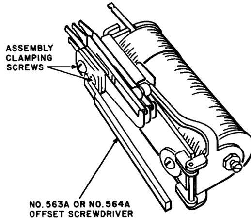
Fig. X—Aligning Contact Springs
