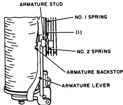
Fig. V—Illustrating Armature Stud Requirement
