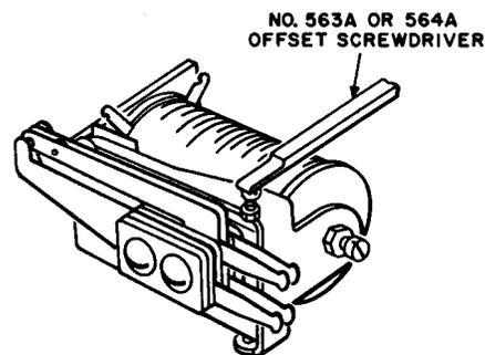
Fig. Y—Adjusting for Armature Movement
