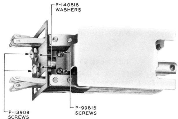
Fig. 2 - Y-type Relay - Side View
