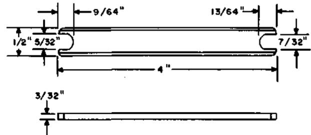
5/32- and 7/32-inch open double-end flat wrench. Replaces the 75 tool. For general use.
