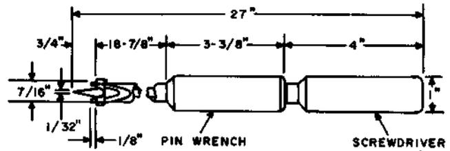
Combination pin wrench and screwdriver. Replaces the 22 tool. For use on jack fasteners.
