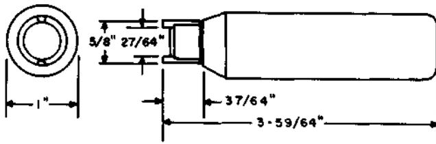
Pin wrench. Replaces the 82 tool. For use on 223-type keys.
