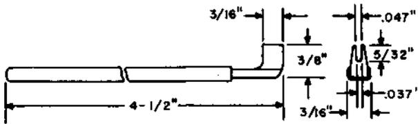
Spring adjuster. Replaces the 50 and 327 tools. For use on 111 and similar-type relays and elevator apparatus.
