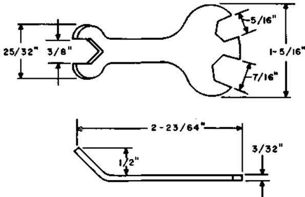
5/16-, 3/8-, and 7/16-inch hex. open-end wrench. For use on General Electric Company voltage regulators.
