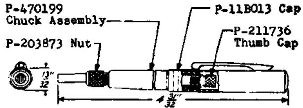
Contact burnisher holder having a chuck for mounting 266-type tools, a magazine for containing these tools and a removable cap with pocket clip. Five No. 266E and 6 No. 266C tools are furnished with the No. 265C tool.
