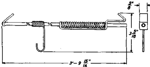
Portable lamp fixture. An adjustable support arranged to attach to channels or angles of panel type frames. Adjustable for different width frames.
