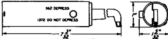
Test tool. 562 ohms and 1372 ohms.
