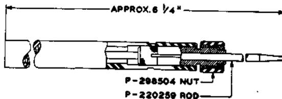
Test pick. This tool may be connected to a No. 893 cord by means of a 360-type tool.
