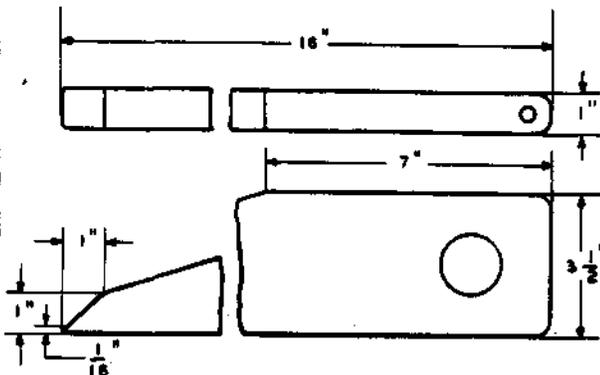
Hardwood wedge. The slanted end of the tool may be cut to any required length.
