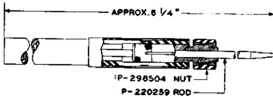
Test Pick. Same as 411A except that at the chuck end the handle is covered with insulating tubing which insulates a metal ring around the handle.
