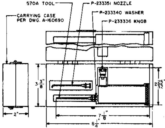
Oil gun. Designed to discharge oil in definite limited quantities. Furnished with a wooden carrying case and two nozzles, one straight and one curved.
