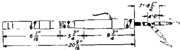
Multiple inspection lamp. Equipped with a W2AL cord, two No. 360A tools and two test clips. Arranged for but not furnished with an A2 lamp. A B1 lamp may be used if greater illumination is required.
