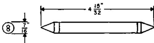
Line switch test tool. Resistance 1100 ohms for 472A, 1300 ohms for 472B, and 1650 ohms for 472C.
