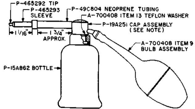
Note - When ordering P-19A251 cap assembly also order one A-700408 Item 13 Teflon washer. Thread washer on cap before mounting cap on bottle.
