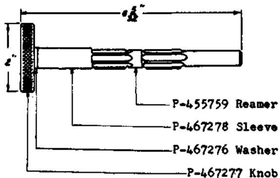
Reamer. This tool forms part of the No.1000A tool kit. For use in replacing bushings on reciprocating bar type interrupters.
