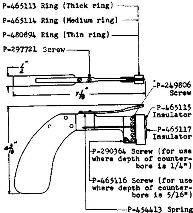
Note: When P-454413 spring is ordered for use on the earlier type tool on which the spring is secured by flat head screws order in addition two P-297721 screws for attaching the spring to the tool. The present type spring is not countersunk for flat head screws.
