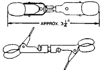
Cord Support. This tool forms part of the J94724 contact closure test set.
