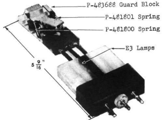
Contact Closure Indicator. This tool forms part of the J94724 contact closure test set.
