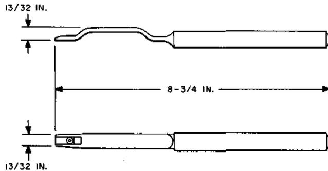
**Relay hinge-bracket adjuster**
