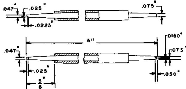
Contact aligning tool
