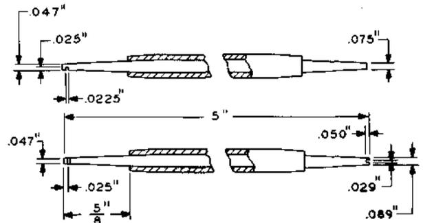
Contact aligning tool
