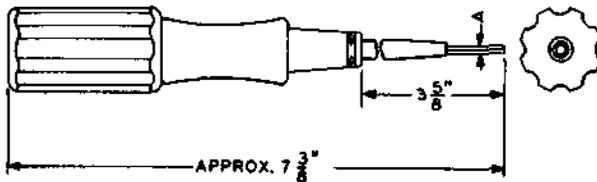
Wrenches for hexagonal socket-head screws
