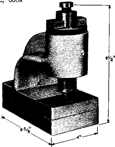
Hole-enlarging punch and die assembly
