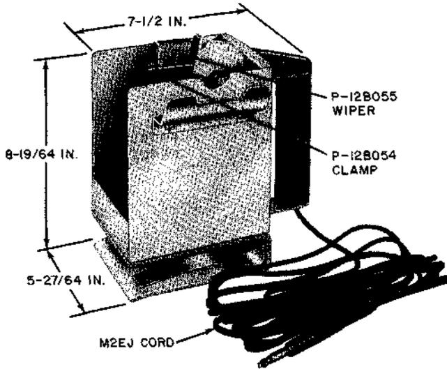
This tool, together with 708A, 708B, 709A and 709B tools, replaces the KS-13503 Compound Remover.
