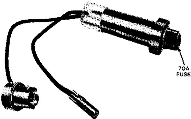
Test battery pickup for use with 70-type fuse mountings.
