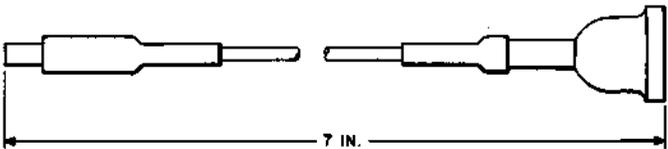
Clutch pin probe, scope adapter. Similar to the 736A tool, except that it has an adapter to connect to an oscilloscope. For use in the No. 101 ESS.
