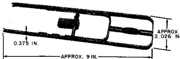
Circuit pack extractor. For use in extracting Amplas circuit packages from mounted KS-19437 connectors in common systems.
