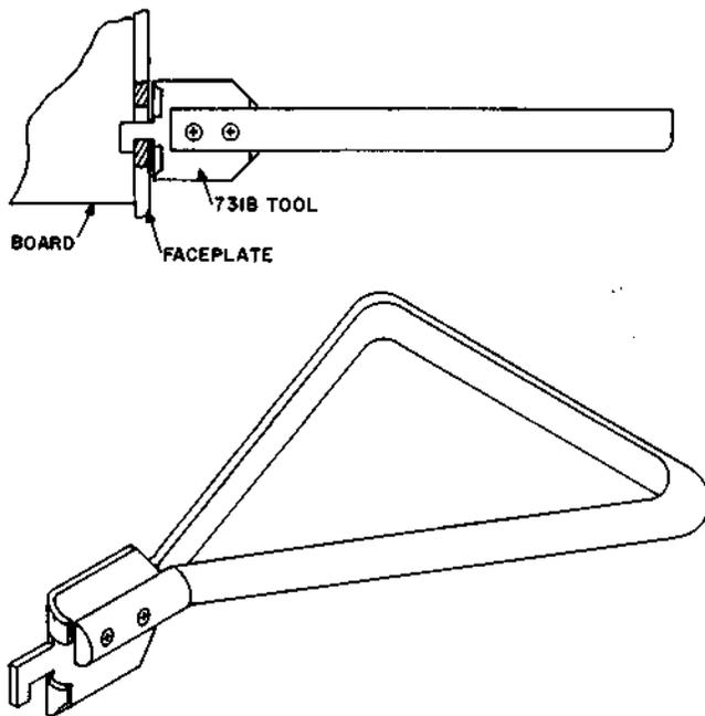
Card puller. For use in extracting packages from the switch unit or control unit. For use in the No. 101 ESS.
