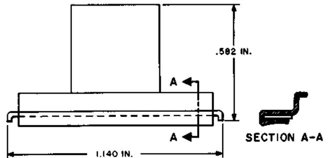
Insulator. For use in insulating levels 1 through 9 of the 9A commutator of step-by-step switches in No. 1, 350, and 355A step-by-step central offices during test procedures.
