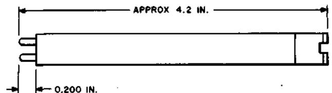
Shorting clip. For use when installing and removing shorting clip in the No. 101 ESS.
